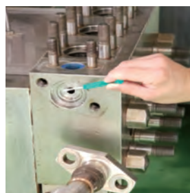
High-pressure pump outlets
