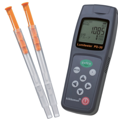
Photo 2: ATP test instrument "Lumitester PD-30" (right) and its reagent "LuciPac Pen"(left) manufactured by Kikkoman Biochemifa Company.
